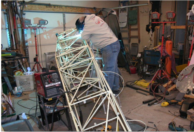
Larry Mueller welding on the Bakeng Deuce fuselage.
